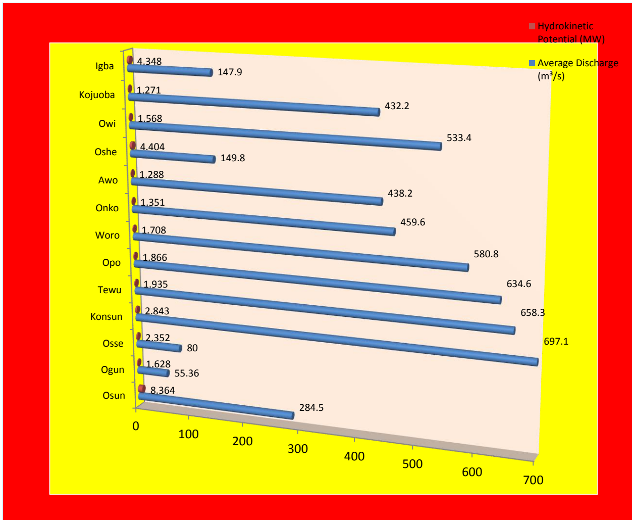
Figure 5: Average Discharge and Hydrokinetic Potential of Selected Basin in the Upper Ogun Basin Nigeria
